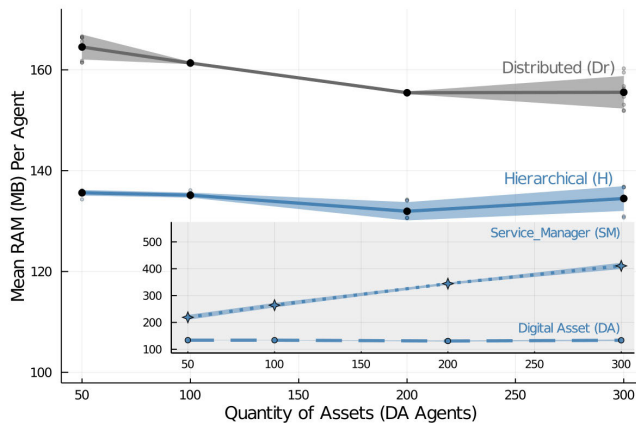
FIGURE 12. Mean RAM usage for two architectures with up to 300 DA agents. The inset shows mean usage per type of agent in the Hierarchical architecture.
