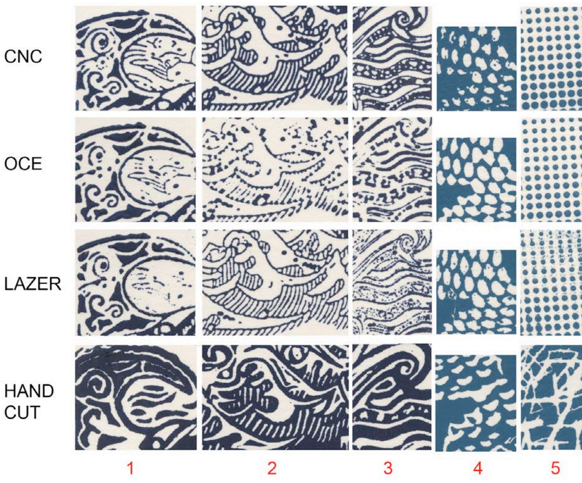
Figure 7: (middle) Details of the fabricated printing plates. The plates are inked, which highlight the differences. Processes from left to right: laser cut, CNC milled, 2.5D print, and hand cut lino.
