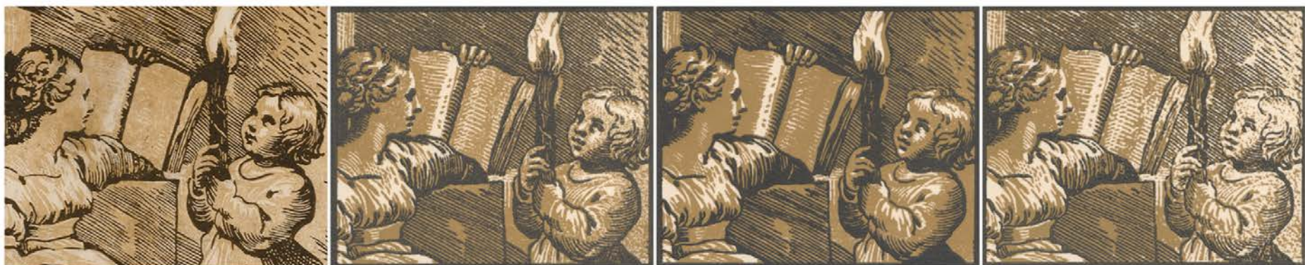
Figure 1: Illustrations of Sibyl Reading, “Lighted by Child with a Torch.” From left to right: source image, laser cut, CNC milled, and 2.5D print.
