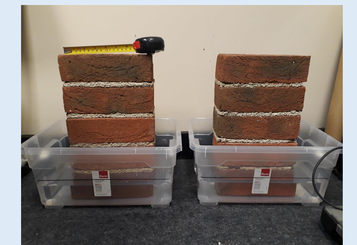
Figure 6: Submersion experiment set-up
