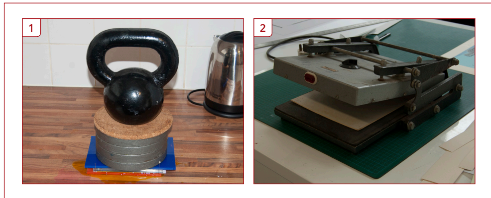
Figure 4.65 1) Makeshift printing press using platen and weights 2) Kennet Dry mount press suitable for printing Woodburytypes
