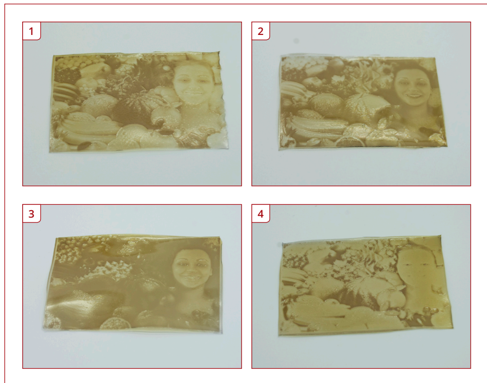
Figure 4.75 Complete set of colour separations for Woodburytype printing 1) Cyan separation 2) Magenta separation 3) Yellow separation 4) Black separation
