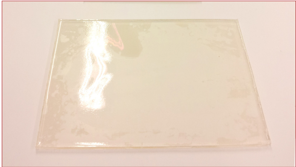
Figure 4.15 Gelating tissue cast at 210mm x 297mm (A4) x 5mm thickness before the drying stage
