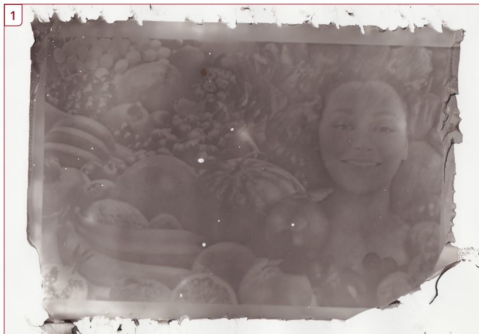
Figure 4.70 Woodburytype print of the test image pulled from a lead plate. Notice the mottled edges
