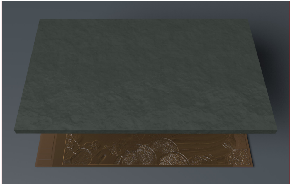
Figure 3.10 A billet of lead is pressed onto the dried gelatine tissue with a lot of even force.
