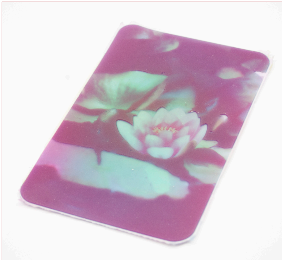
Figure 6.35 3 Colour print released from printing plates and printed into a white silicone substrate.
