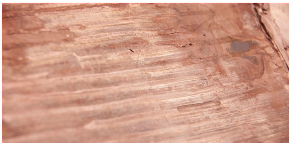
Figure 4.46 Partial detail of relief did build an electrodeposit, however relief was destroyed before electroforming process completed
