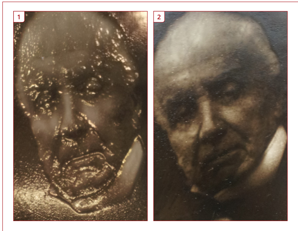
Figure 4.69 1) Woodburytype print wet and in relief 2) Woodburytype print dry and with shrunken relief.
