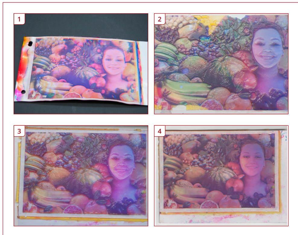
Figure 6.56 1) Printed results using the pin registration system. Notice the right hand side of the print where the separation layers have moved and the substrate surface is badly warped due to moisture. 2) Fence registration system used with rigid mount board substrate. Notice the tears in separation layers at the top of the image due to suction caused in removing the print. 3) Successful registration of the print and no tearing due to the inversion of the printing plate before removing from the print. Notice the right handside of the plate where the temperature was not correct and the cyan layer set too early. 4) The same image presented in 3, however it is now fully dried. Notice the vast reduction in print height and the sharp edge of the print boundary before the excess overspill in yellow.
