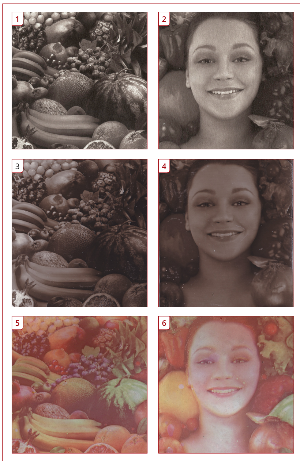
Figure 6.84 Comparison of three continuous tone processes using the same source image. 1-2) Carbon Print. 3-4) Digital Woodburytype, 5-6) Digital 3 Colour Woodburytype
