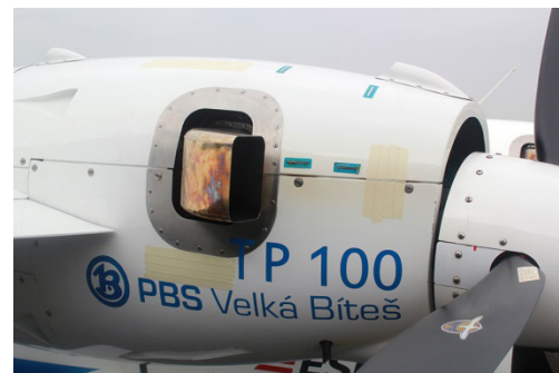
Fig. 16 The exhaust pipe on left engine of aircraft AM-11 OKRA
