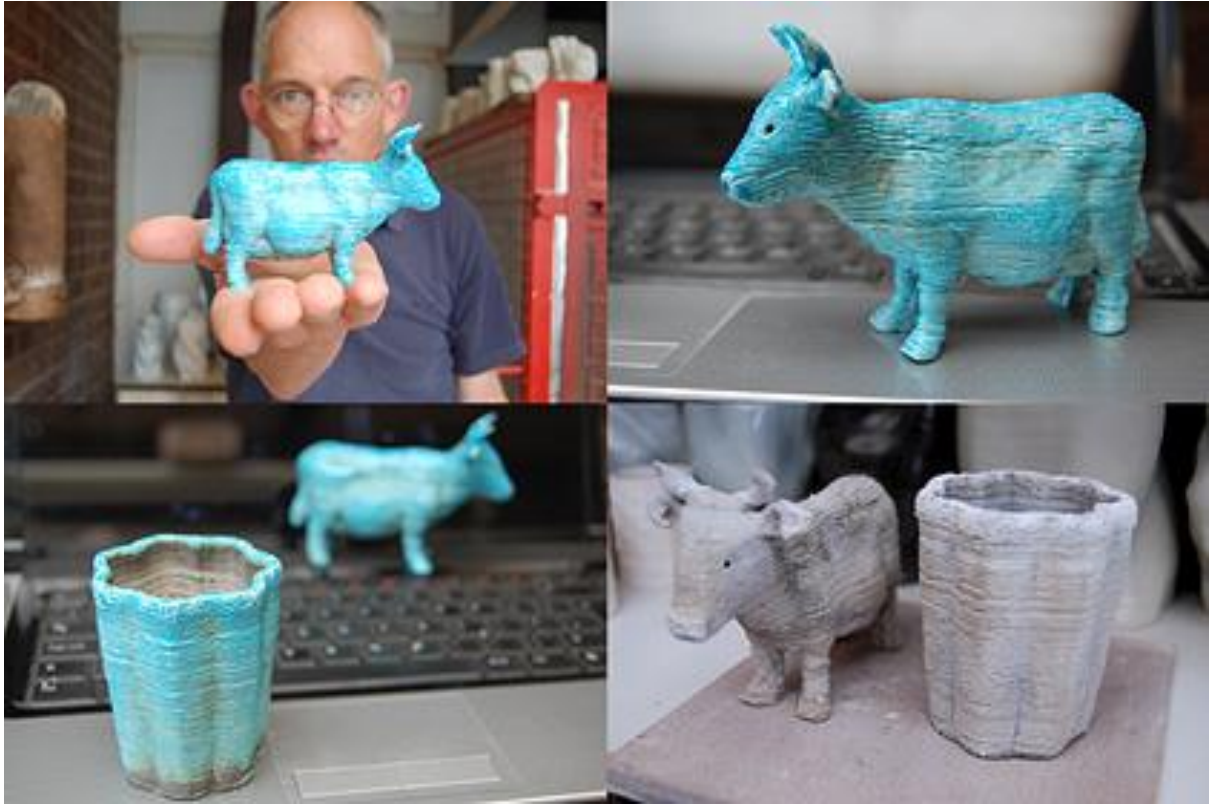
Figure 37: Objects formed through faience 3D paste extrusion (2012)
