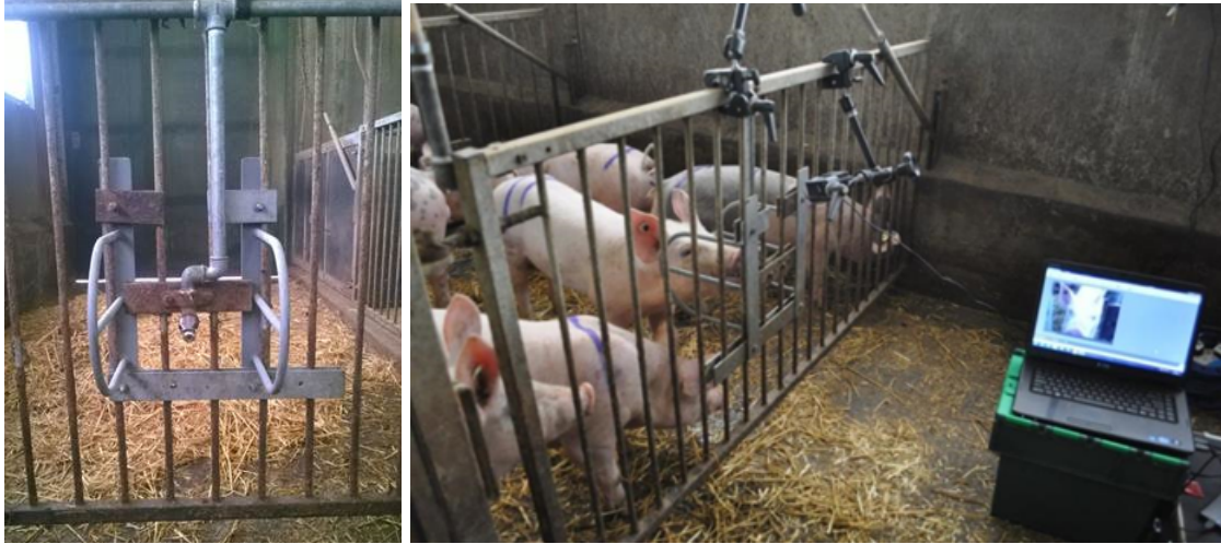
Figure 2: Photographs showing the modified drinking nipple (left) and the arrangement of the webcam behind it (right).
