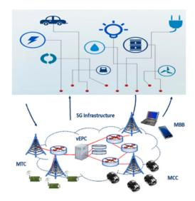
Figure 7: Example of 5G-IoT architecture [7, 12]
