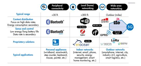
Figure 6: Technologies associated with 5G-IoT [47]
