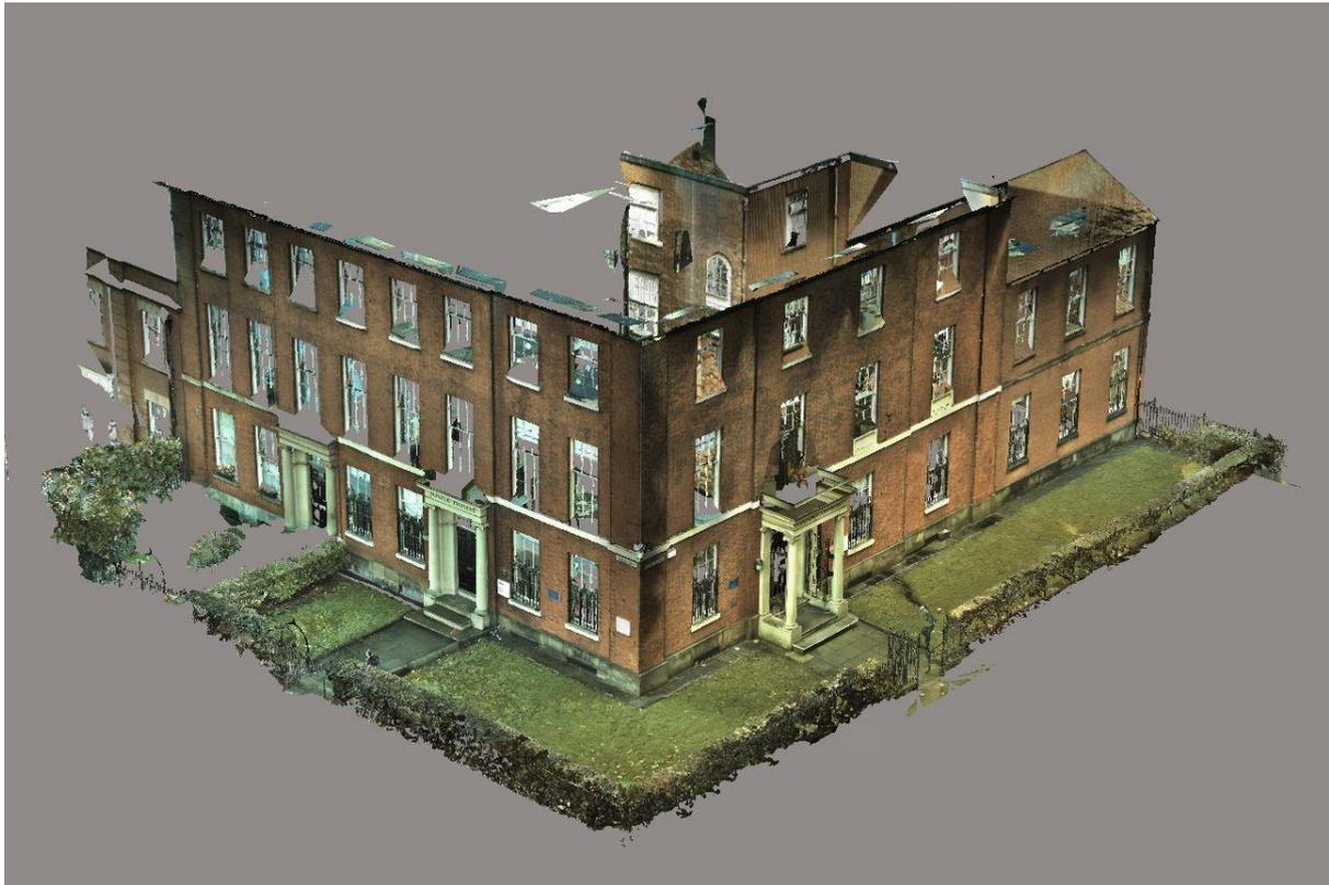
**Figure 7: 3D mesh generated from 9 scans of Joule House.**
