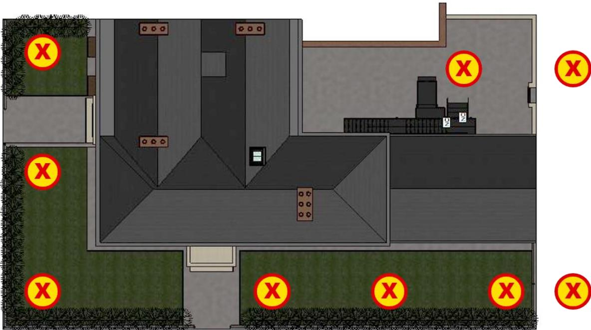
**Figure 5: Scan Station locations during the laser scan of Joule House.**
