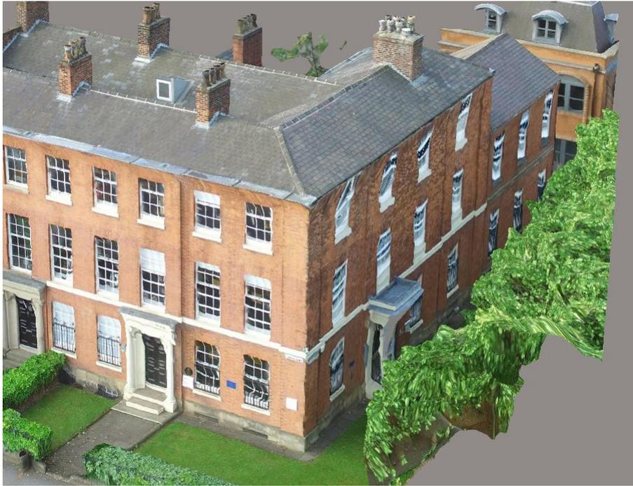
**Figure 10: 3D mesh of Joule House generated from aerial photogrammetry.**
