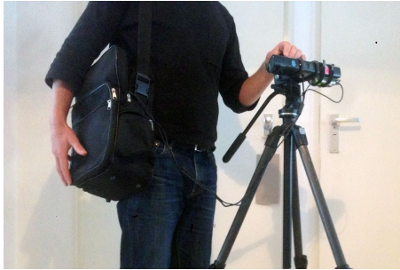
Figure 3: Portable hand-built Volca experiment rig with USB button interface for eternal control, illustrating Kinect sensor array on tripod rather than hand held. with CPU, batteries controls .etc are carried in shoulder bag.
