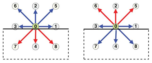
Figure 2: The bounce-back boundaries principle in a D2Q9 lattice.
