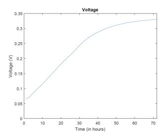
Figure 9: MFC output voltage over time in hourly intervals.
