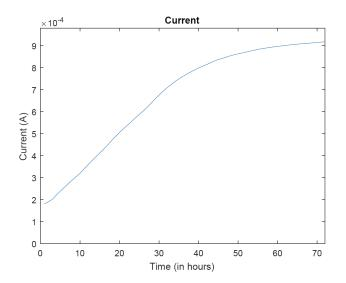
Figure 10: MFC output current over time in hourly intervals.
