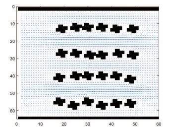
Figure 4: Flow field in the anode without a developed biofilm.
