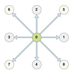
Figure 1: The D2Q9 lattice.
