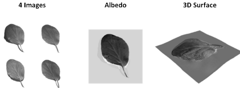
Fig. 4. Four images captured using Fig. 3 rig, which are combined with a lighting model to generate the albedo 2D leaf data and the 3D leaf surface.
