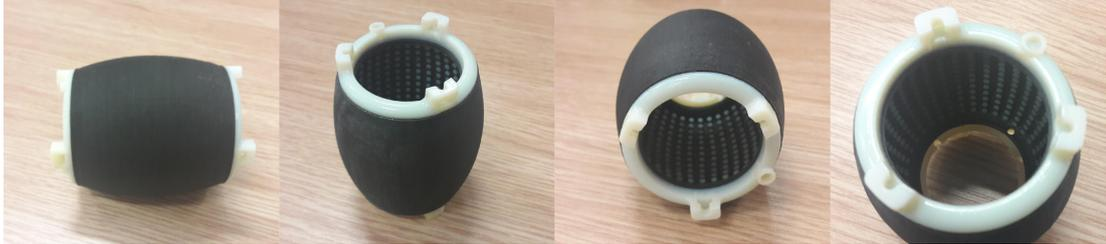
Figure 3.12: Complete 3D printed cylindrical Tactip skin. Printed from two separate materials, solid vero white, and soft tango black.
