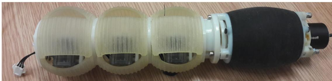
Figure 5.17: Built assembly of integrated of locomotion and sensing modules.
