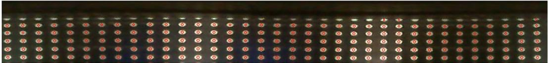
Figure 3.18: Unwrapped 360° panoramic image capture with identified pin positions.
