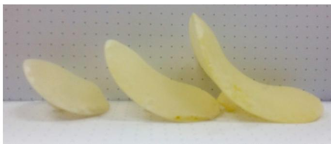
Figure 4.12: Soft test pieces spread circumferentially around sensor,  $60^\circ$ ,  $90^\circ$  and  $120^\circ$  left to right. Soft lumps are made from cast Platsil 7315 rubber silicone.
