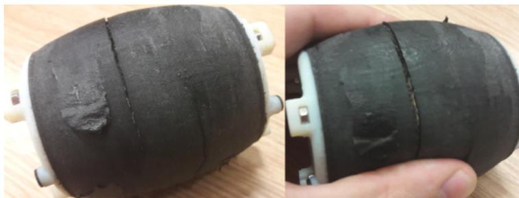
Figure 3.15: View of fractured 3D printed skin that occurs much quicker than cast silicone skin. The fatigue is caused from repeated contact and friction with another surface where over time the integrity of the flexible rubber breaks down.
