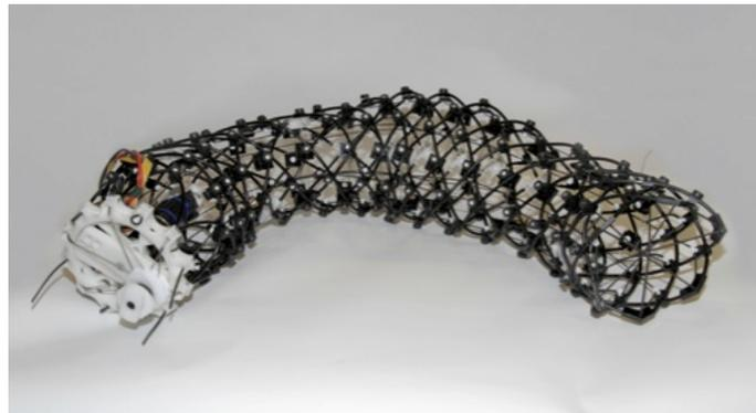
Figure 2.17: Peristaltic worm robot, Boxerbaum 2012. ©2012 IEEE.
