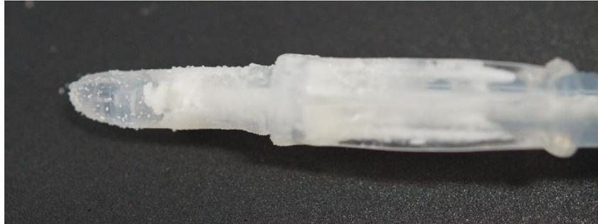
**Figure 50. Photograph of a blocked catheter** removed from the *in vitro* bladder model system. Crystalline deposits have completely occluded the eye hole and are visible on the tip and balloon. Cuffing, the creases and ridges that form as the retention balloon fails to return to its original size, is also evident.
