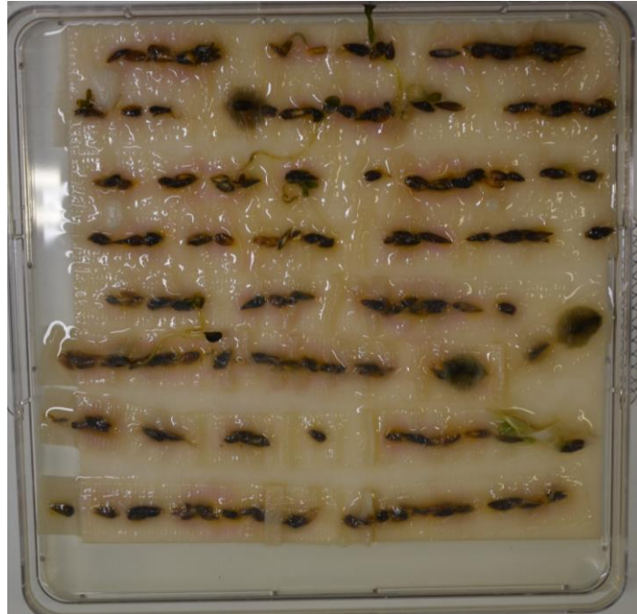
Figure 8.1, An image of the Zinnia Paper A specimen, captured on day 15. The dark patches around the seeds are the beginning of the rotting process.
