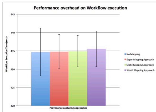
Figure 22: Effect of different provenance collection approaches on the workflow execution performance.
