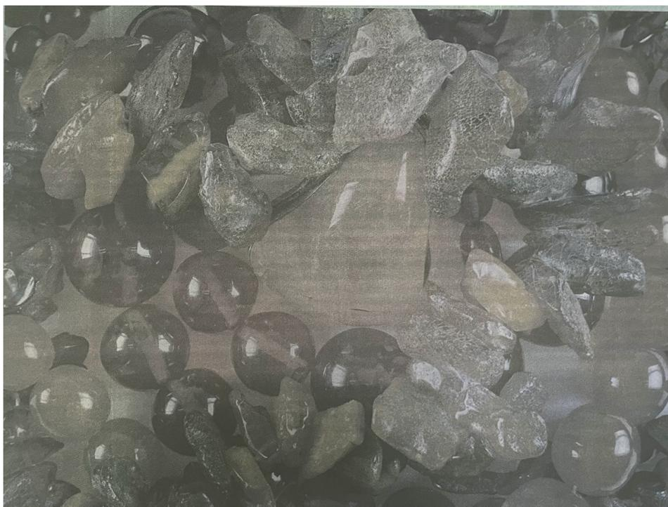
**Figure A11.** 25LPI, offset litho, Spectraval™ pigments, R = 2× pass, G = 3× pass, B = 4× pass black Plike, film negative, print size: 600 mm × 450 mm.
