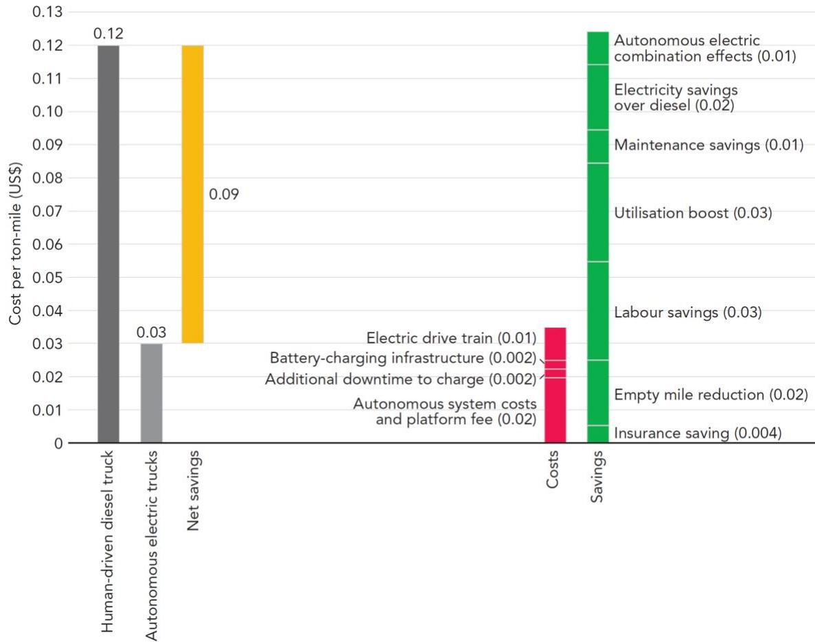
**Figure 13: Electric vehicle savings and autonomous vehicle savings<sup>29</sup>**
