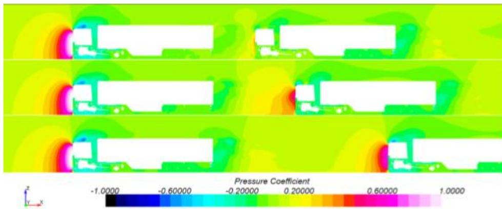
**Figure 6: Simulation of air pressure for two trucks for different inter-vehicle distances**
