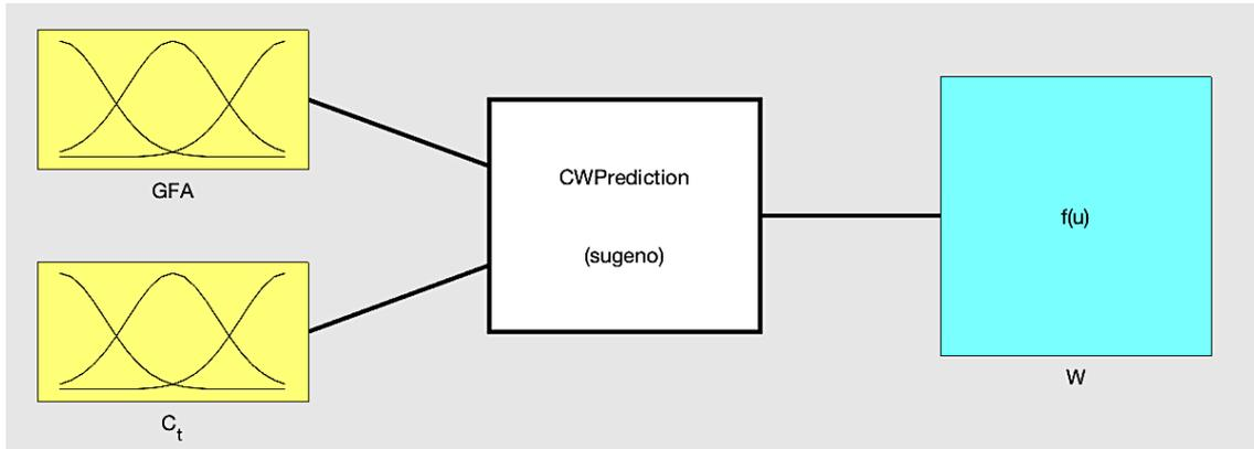
355 *Figure 6: Block diagram of the final ANFIS model*
