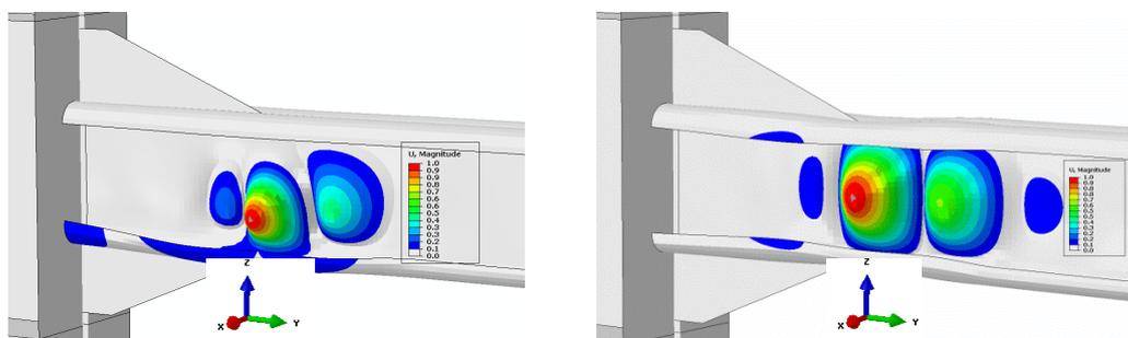
**Fig. 5:** First buckling mode shape in the cases of: (a) monotonic load (b) cyclic load.
