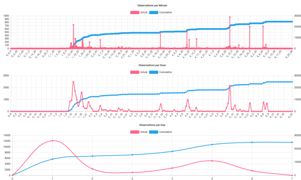
Fig. 3: Aligned time-series plots at different temporal scales to assess the targeted phishing impact, based on number of suspicious e-mail observations. Top: Per minute. Middle: Per hour. Bottom: Per Day
