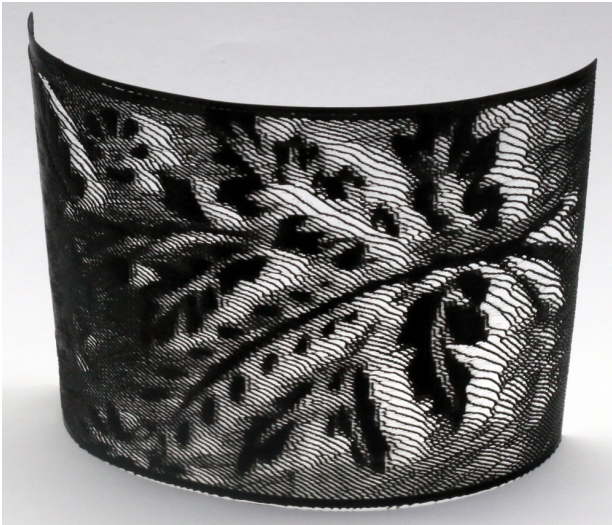
Figure 5. An example of 'lace' like aesthetic created by modulated nozzle velocity.
