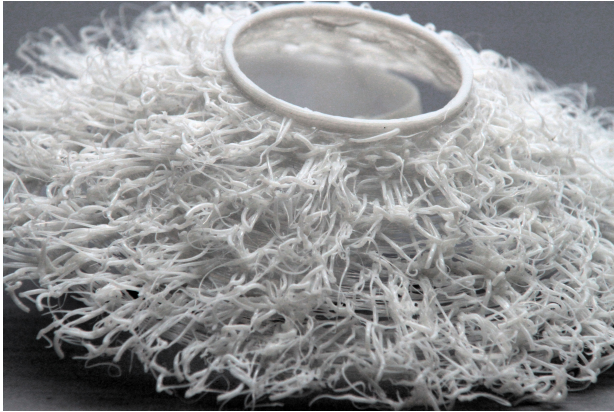
Figure 9. A 'hairy' texture, which can be printed consistently yet retains a unique character bestowed by the material medium itself.
