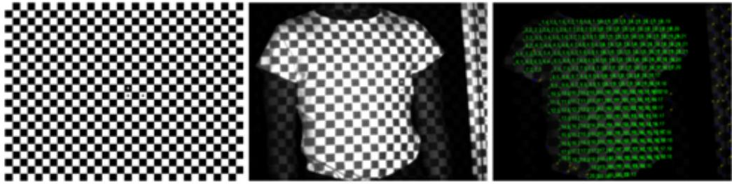
Figure 2.7: SLP projected pattern and corner detection
