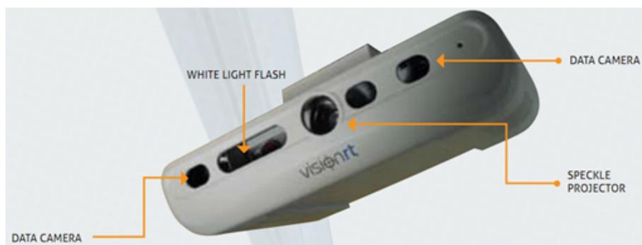
Figure 2.14: AlignRT breathing monitoring system by Vision RT UK.
