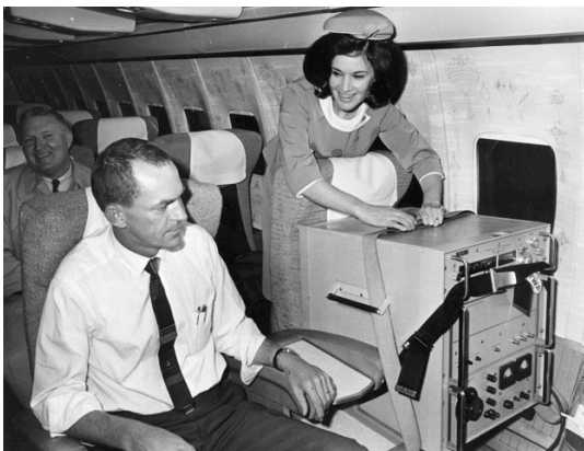
Figure 1: A caesium beam timepiece used in the U.S. space program occupies a first-class seat aboard a TWA flight from London to Washington on Nov. 23, 1966. This formed part of the famous Hafele-Keating experiment published in 1972.
