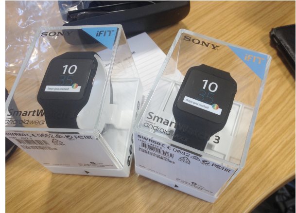
Figure 11: Sony SmartWatch 3 model SWR50 chosen for testing contains in-built GPS capability which allows our application to work without the necessity of a tethered Android phone.
