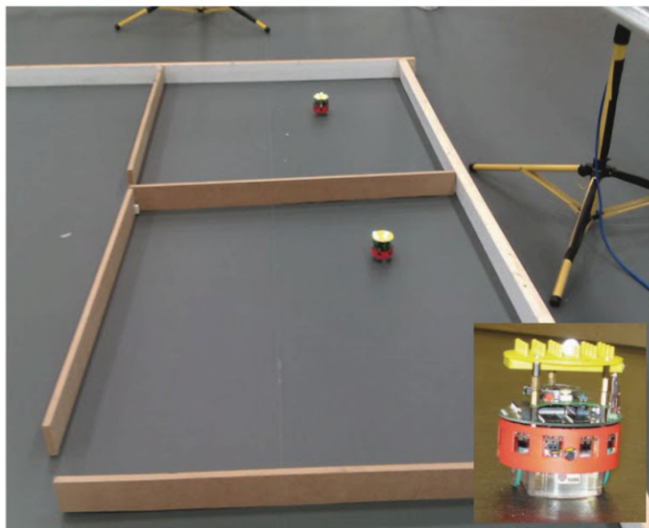
Figure 10. The work areas of the two e-puck robots used in the imitation-enhanced reinforcement learning experiment. Note the small gaps in the bottom left of each area.
