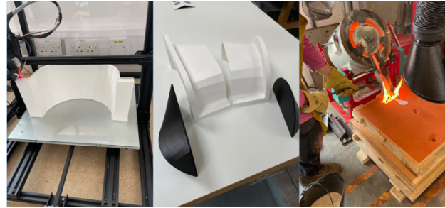
Figure 1: Images from the workflow of the investigation, foundry pattern being printed via FDM, two-part 3D printed pattern with separate end-caps, molten aluminum being poured (Photos by T Jorgensen 2020).
