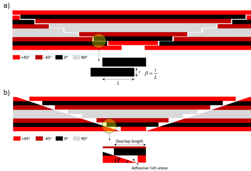
Figure 2: Examples of laminated composite repair schemes, a) stepped scarf repair and b) ramped scarf repair as seen in the literature
