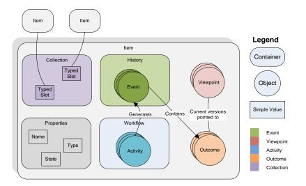
Figure 1. The components of an Item in CRISTAL
