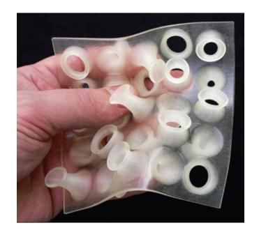
Photopolymer model made using the EnvisionTEC Perfactory rapid prototyping system Photopolymer model made using the Objet Geometries PolyJet 3D printing system TangoPlus rubber-like resin
