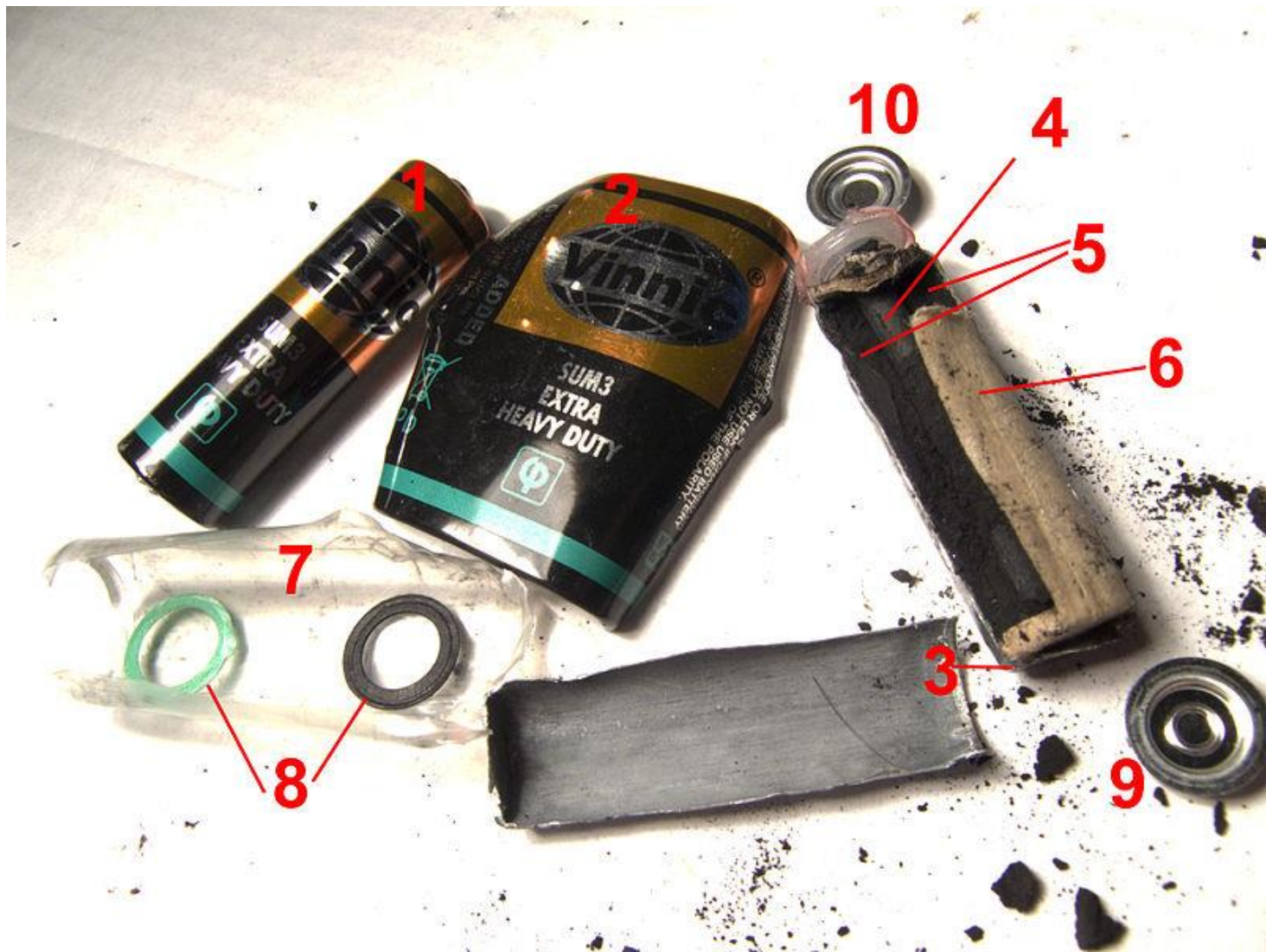
Figure 1. Disassembled zinc chloride cell (similar to zinc carbon cell). 1:entire cell, 2:steel casing, 3:zinc negative electrode, 4:carbon rod , 5:positive electrode (Manganese dioxide mixed with carbon powder and electrolyte), 6:paper separator, 7:polyethylene leak proof isolation, 8:sealing rings, 9-negative terminal, 10-positive terminal (originally connected to carbon rod)
