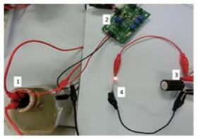
Fig.1. The experimental set-up during the 7-day operation continuously powering a LED (1-MFC, 2-TI energy harvester, 3-capacitor, 4- LED)
