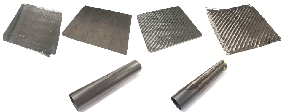
Figure 6. (Top): Photographs of the four planar samples: from left, these are Cured UD, dry UD, cured woven and dry woven. (Bottom): Tubular samples: from left, these are cured UD and dry UD. The dry UD tube simply comprises the cured piece wrapped in dry UD fibres.
