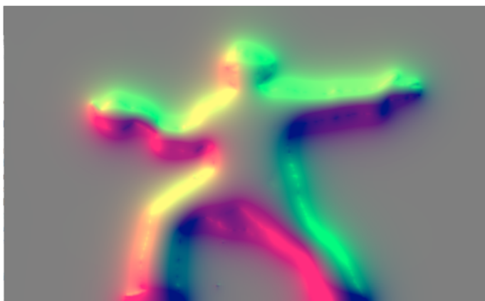
Figure 5 - Force topology map of the human form. Gray indicates a gradient of zero. The intensity of each color is related to the magnitude of the local force vector on the depth image. Color choice has been selected to effectively illustrate depth
