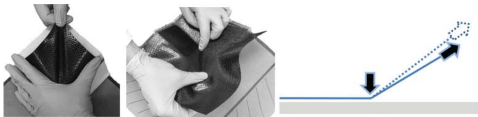
Figure 10 (Left) 'Tension-secured shearing' in use during Task 6. In this example, the left hand at the bottom of the picture secures the prepreg, while the right hand applies tension. (Centre) 'Tension secured shearing' in use on Task 8, the left hand at the top of the picture is securing while the right hand is applying the tension. (Right) Schematic force diagram of technique (not to scale)
