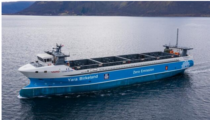
Fig. 3. Fully battery powered ship Yara Birkeland. (Source: Yara International)
