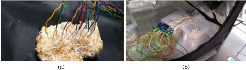
Figure 1: Experimental setup. (a) Exemplar locations of electrodes. (b) Electrode pairs and logging setup in the tent.
