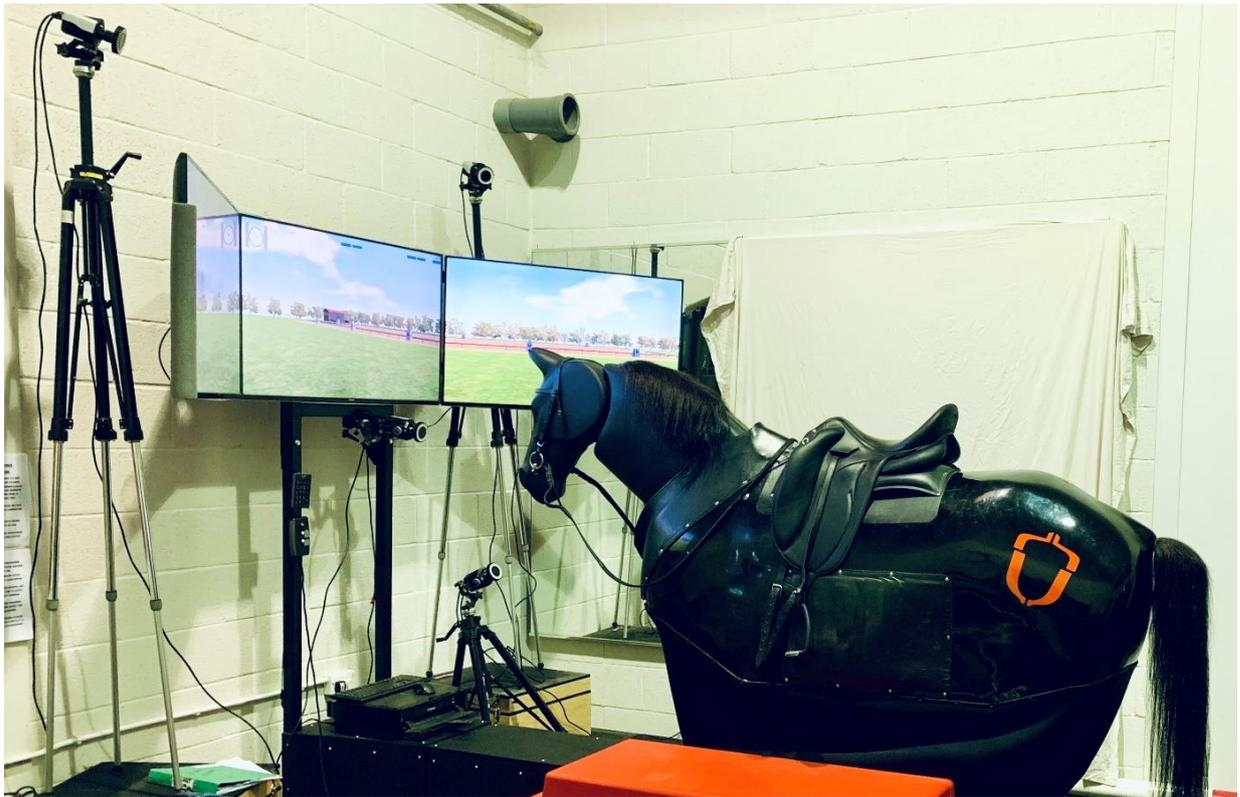
**Figure 3.3.** The riding simulator in Arena Mode with standard saddle and motion capture cameras. Not pictured: motion capture cameras placed to the rear and left side of the simulator.
