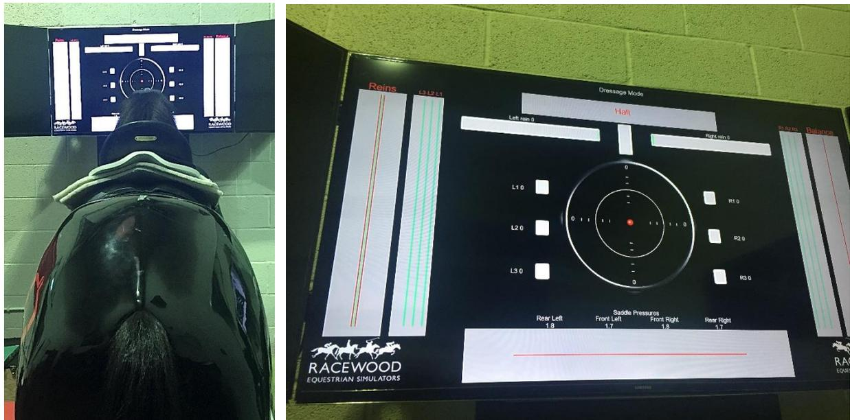
**Figure 3.4.** The riding simulator screens in Instruction Mode. The circle depicts the data from the four pressure sensors located under the saddle. Other bars indicate the leg pressure and rein pressures from the pressure sensors embedded into the side of the riding simulator and at the end of the reins.
