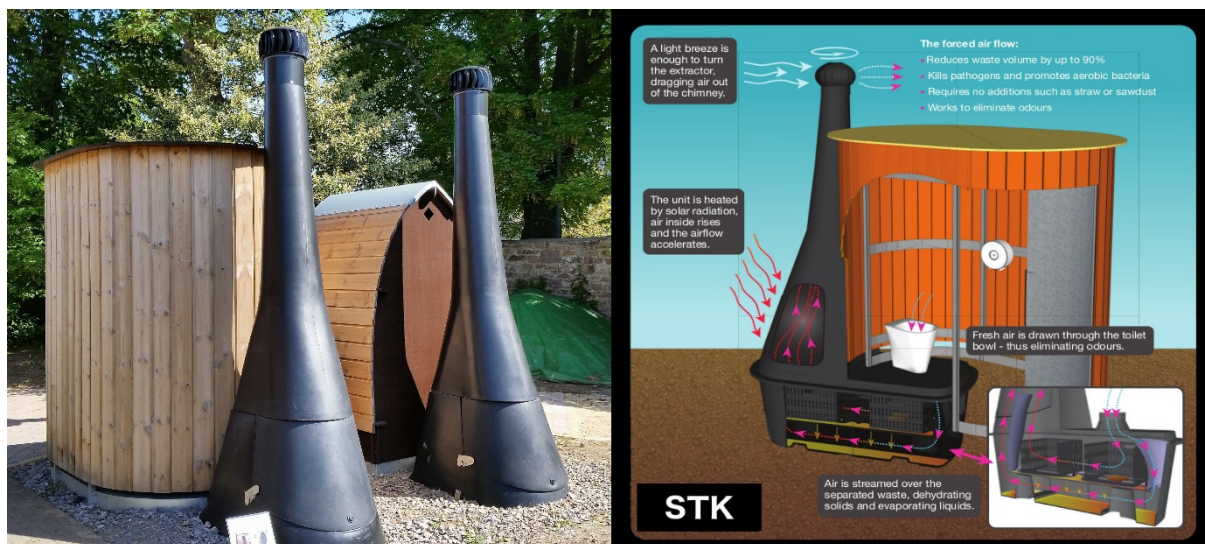
Figure 7. Photograph of composting toilets at University of Bristol Botanic Gardens and diagram showing how the system works. Diagram courtesy WooWoo [91].
