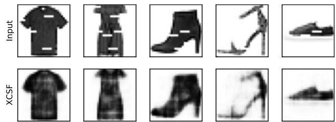
Fig. 7: XCSF reconstruction of samples from MNIST FASHION test set with random cut out after 100000 trials. Training MSE = 0.0082 and P_h = 67.2 .
