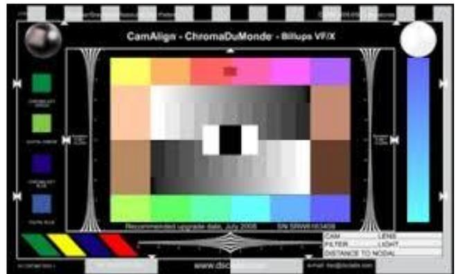
*Set at ISO 400 in sunny exterior (noon March 2017), using a CamAlign ChromaDuMonde chart – a standard camera testchart for cinematography. These tests were done with self-made shim pinhole apertures ranging from diameters of 0.02 to 0.90mm.*
