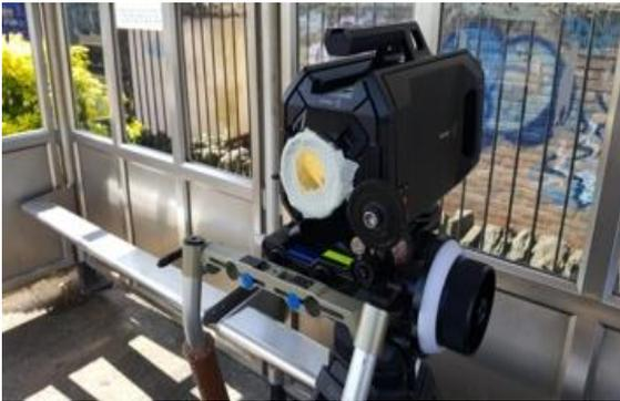
*4K Black Magic cinematography camera with self-produced multiple pinhole disc (0.35mm) 800 ISO (noon sun, May 2017).*
