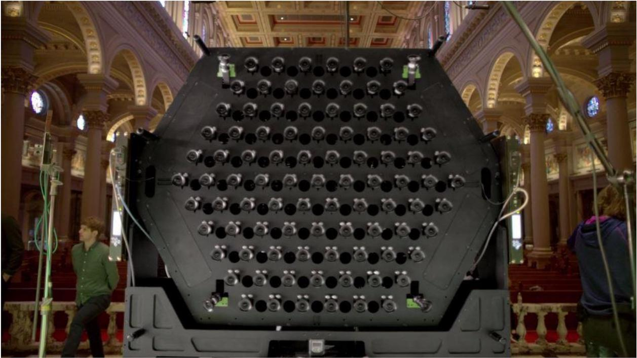
Fig.15: Lytro Immerse Camera with its multi-lens array generating light data which involves a huge amount of post-capture calculation. (Image: Lytro, 2016).
