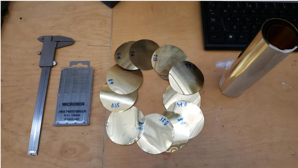
Fig. 21: Making the first test pinhole discs from brass shim sheet (shown in a roll above right)
