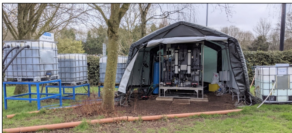
Figure 1. The decentralised drinking water treatment system (PAQUA 1000-D) trialled at the University of the West of England, Bristol.
