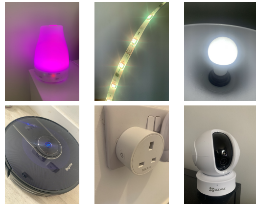
Fig. 4. Consumer devices connected using the Tuya IoT network. Top row: LED Humidifier, LED strip light, LED bulb. Bottom row: Robot vacuum, Power socket, PTZ Camera.
