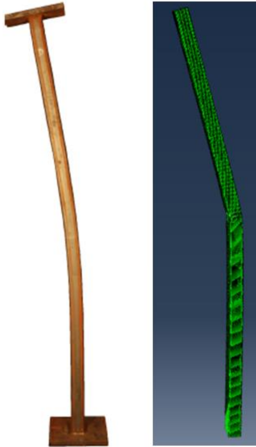
Figure 5: Images of the failure modes from the test specimens (Pauli et al., 2012) and FE simulations for (a) column L6 with a 160 \times 160 \times 5 SHS cross-section and (b) column L10 with a 120 \times 60 \times 3.6 RHS cross-section.
