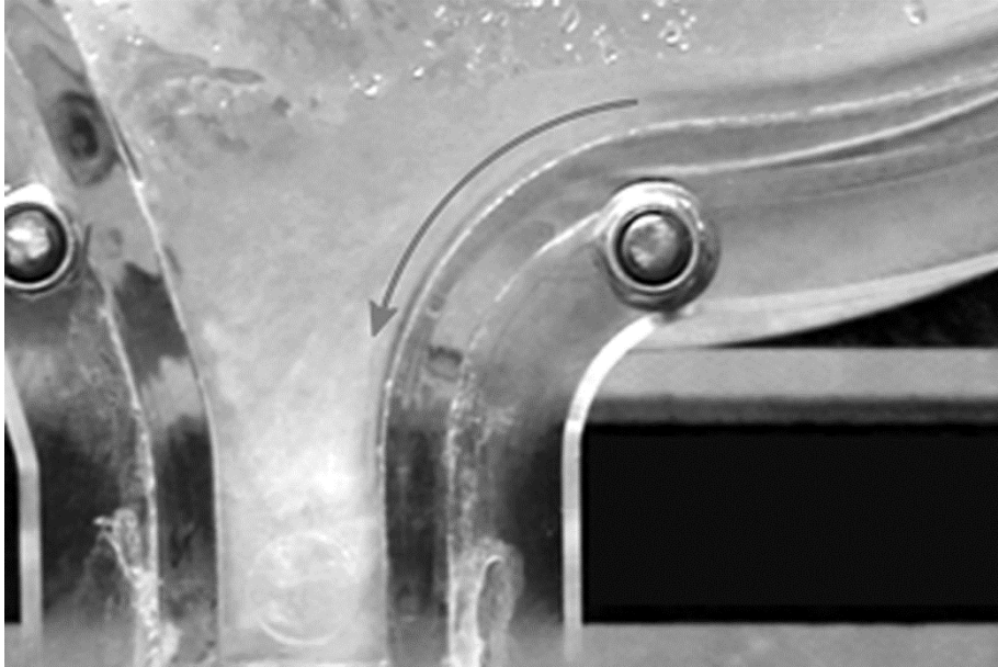
Fig. 15 Gentle sloping upstream wall of CWDS helps incoming flow to stay attached
