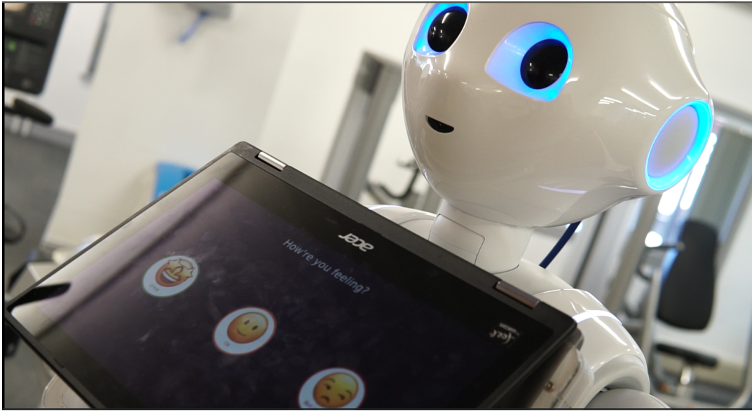
Figure 4.6: The C25K Robot-mounted tablet showing the ‘Check PRE’ action, with the robot’s speech in subtitles and icon-based buttons for the user to respond to its question.
