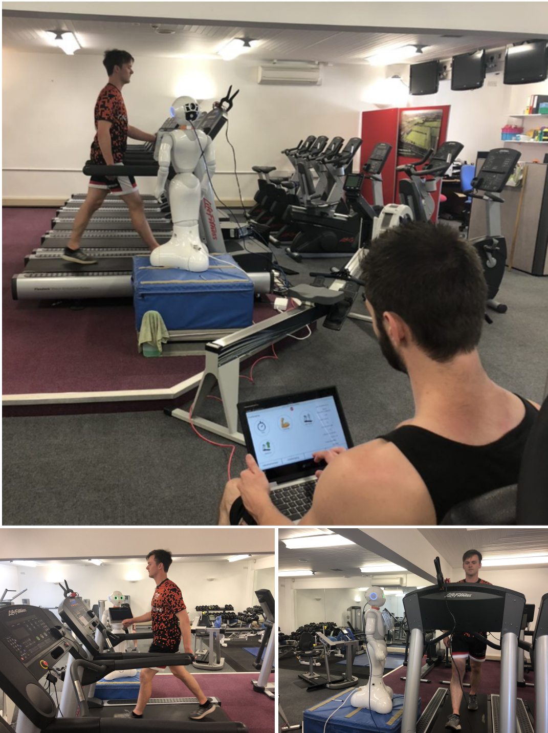
Figure 4.8: Final experimental set-up; photograph of an exercise session undertaken during the study. Shows fitness instructor and robot position with regard to the participant, and the fitness instructor's use of the teaching interface to control/supervise the robot.
