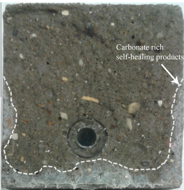
Fig. 8. Typical self-healing materials formation pattern in the cracked cross-section of sample cured under water.
