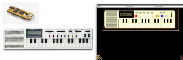
Figure 1: Left is a hacked Casio VL-1 with an Electro Smith's Daisy running a AA Module, emulating a version of the VL-1 audio engine. Right is the same emulation running in AA hosting application.
