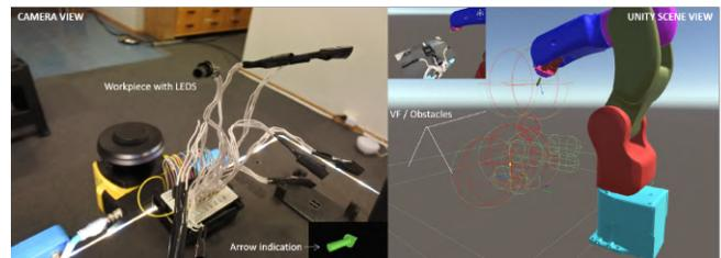
Fig. 7. The 3D arrow used for for the visual feedback in the fourth experiment scenario and the Unity scene view of the obstacles.
