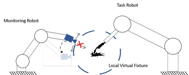
Fig. 1. Conceptual representation of a virtual fixture. The virtual fixture prevents the robot's end-effector from entering a certain forbidden region.
