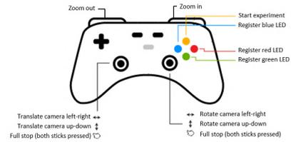
Fig. 6. Input mapping for the joystick used to control the monitoring robot. The commands are from the camera perspective, which corresponds to the robot's TCP.
