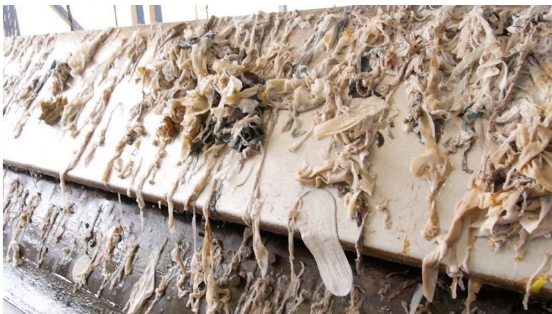
Figure 4. Accumulation: materials that have not degraded or decomposed in the sewers. These will be composted and eventually used for land reclamation.
