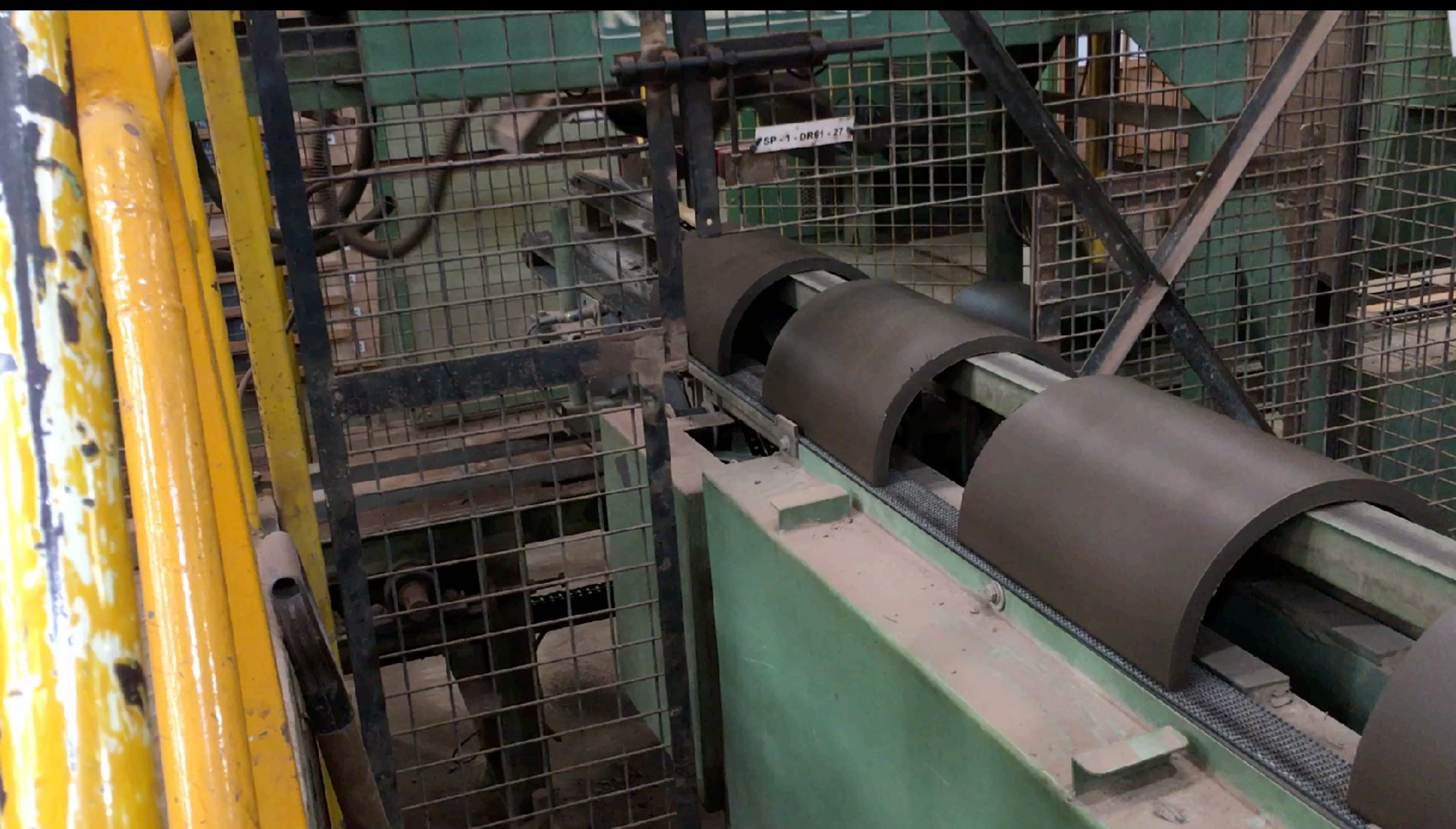
Ridge tile production, Wienerberger Sandtoft site
